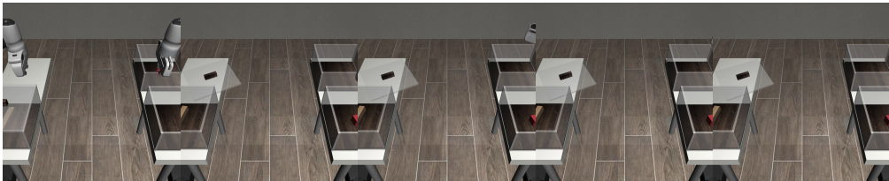
(e) Transport : a bimanual task where two arms coordinate to transfer a hammer from a closed container to a target bin.
