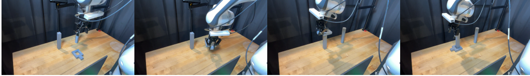
(b) Square : pick up a square nut and place it onto a vertical peg, requiring precise alignment. (external camera view; not used for training)
